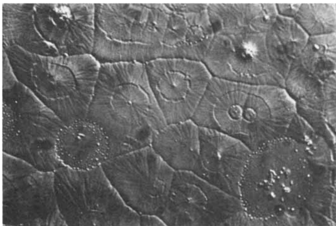
Fig. 4. Examples of polycarbonate spherulites illustrated in Fig. 3 examined by incident interference contrast showing surface markings; mag. \times 900 .
